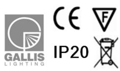
Luminaire without driver: **Protection class III.** Luminaire connected to a driver: **Protection class II.** This fitting is double insulated and should not be connected to ground wire.
