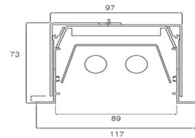
3. Connect the reflector with the electrical parts to the clamp. Be ware to the labeling for grounding. The luminaire is forbidden to function without grounding. **Attention** Make sure that the power is disconnected when installing the luminaire as well as during lamp changing.
